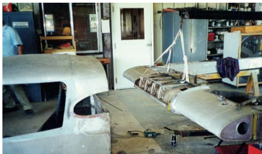
A couple of shots of the structure of the AG-14 during its restoration. You can see the level of skin replacement needed on the fuselage pod.
