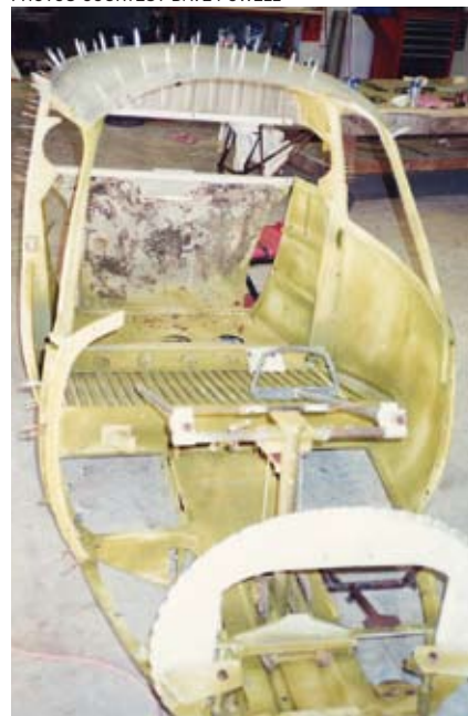
A couple of shots of the structure of the AG-14 during its restoration. You can see the level of skin replacement needed on the fuselage pod.
