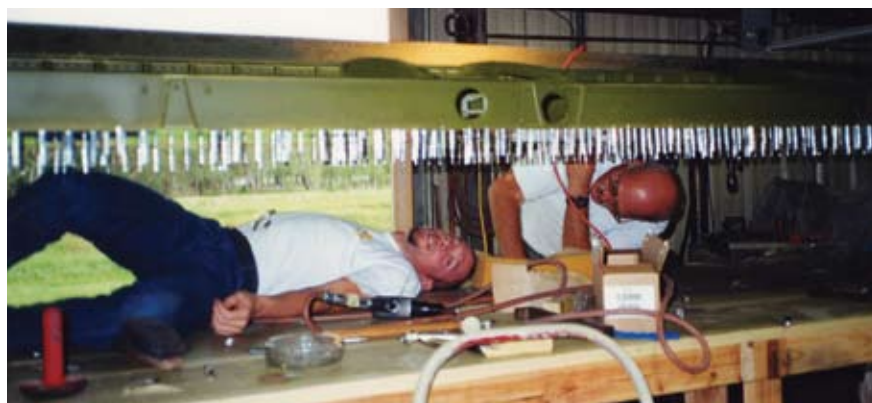
“How bad do you want to restore this airplane?” Thanks in part to a family tie (his dad worked for Anderson-Greenwood), Dave Powell was very motivated to save one of the five airplanes built before the Korean War put a halt to production. All-new skins were required on much of the airframe.
