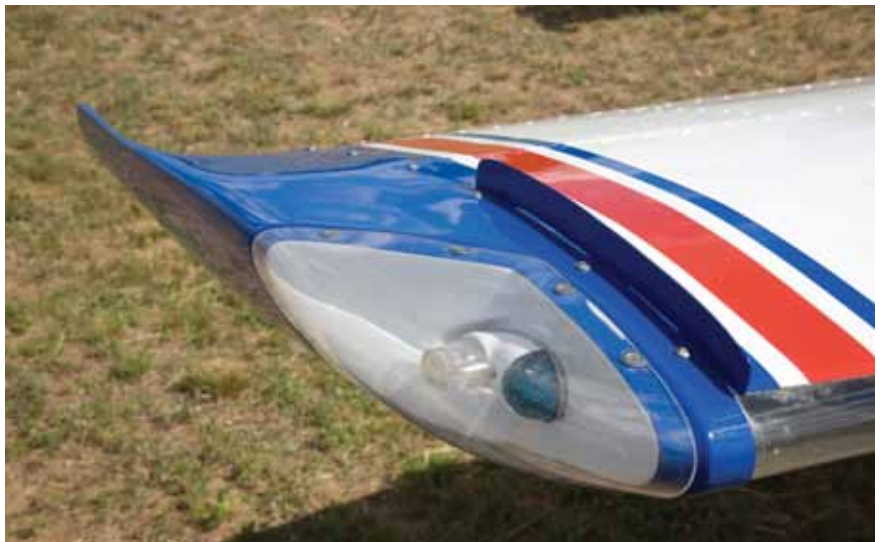
The Johnstone wingtips are specially shaped to flare upwards to allow the wingtip vortices to spill around the wing so that aileron sensitivity is enhanced.
